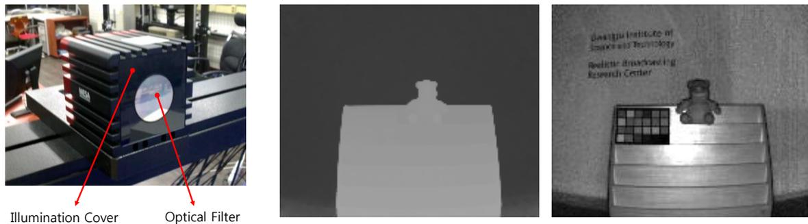
**Figure 2:** Time-of-Flight depth camera – SR4000 and its output depth and intensity images.
